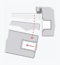
The cover is removable and hides the fixing screws and the adjustment grubs of the magnets. Rotating the grubs increases the working stroke of the magnetic latches and therefore the force of attraction between the sash part and the frame.
