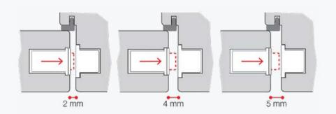
When the door is open, the magnets retract and stay flush with the forend, giving a minimal design to the door and avoiding problems caused by any protrusion.
