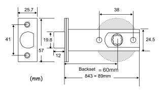
Models L T843 Tubular Latch has a unique design - requiring only 28 degrees, both clockwise and counter-clockwise rotations on either side to retract the Bolt.
